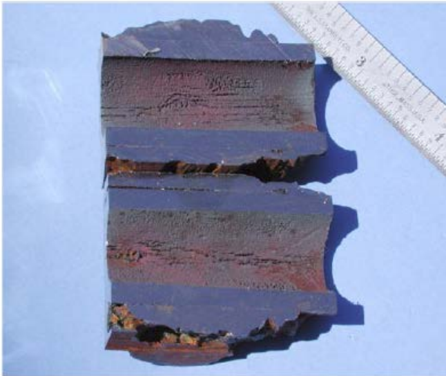
Boiler tube corrosion
